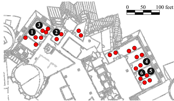
FIGURE 5-19—Experimental Zigbee testbed layout: there are 31 nodes in total, spread over 11 rooms in an indoor office environment. Each unnumbered dot indicates one of 25 Zigbee nodes. The six software defined radio nodes are shown dark, labeled with numbers.
