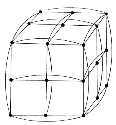
Unfortunately packaging suggested by the above diagram requires a large number of very long wires between opposite faces. Richard Zippel has developed a very clever way to package the Hypertorus topology so that essentially no long wires are required. Below we show the connections for a 4 x 4 two dimensional Cartesian hypertorus.
