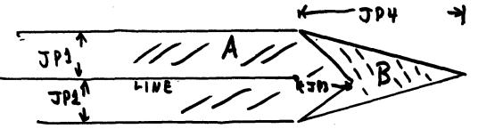
If any point of Q1 Q2 lies within region "A", or if either end point Q1 or Q2 lies within region "B", then a link from P1 P2 to Q1 Q2 is made. By this is meant that a "link" is added to the list on (INFO N 2), where N is the serial number of the segment P1 P2.
