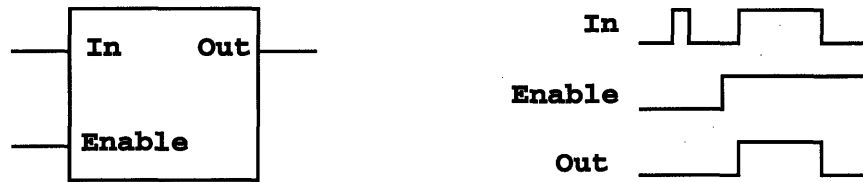
Figure 3-5 Example input waveforms and output waveform for a latch.
