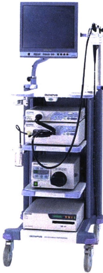
Figure 1.2: A modern day monoscope based endoscopic system complete with HDTV display, fiber-optic light delivery mechanism and a fiber optic data transmission system for the captured images
