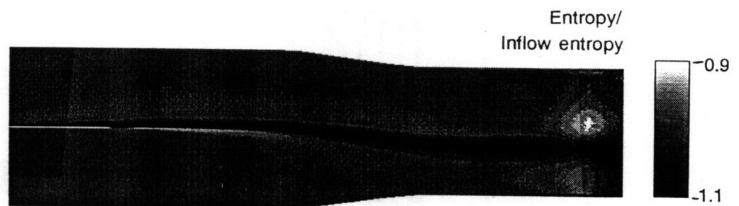
Figure 3-33 Entropy profile of flat plate with combined supersonic/subsonic boundary conditions (Inlet Mach number of 0.26, 1.2)
