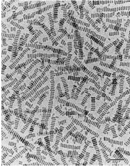
Figure 1 TEM image showing ordered chains of prismatic BaCrO 4 nanoparticles. The nanoparticles were prepared in AOT microemulsions at [Ba 2+ ]:[CrO 4 2- ] molar ratio ≈1 and w = 10. Scale bar = 50 nm.
