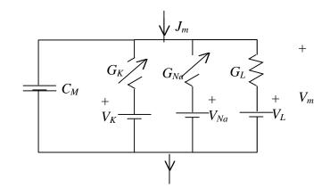
Potassium and Sodium conductance depend on the membrane voltage. Vk and Vna do not change with an AP since very little ions are actually transported...
