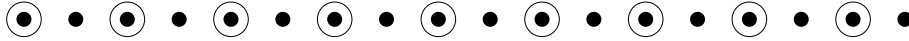
Figure 1: Decimation RG for 1D Ising model. The spins on one family of sites are summed over to obtain an effective Hamiltonian for remaining sites.
