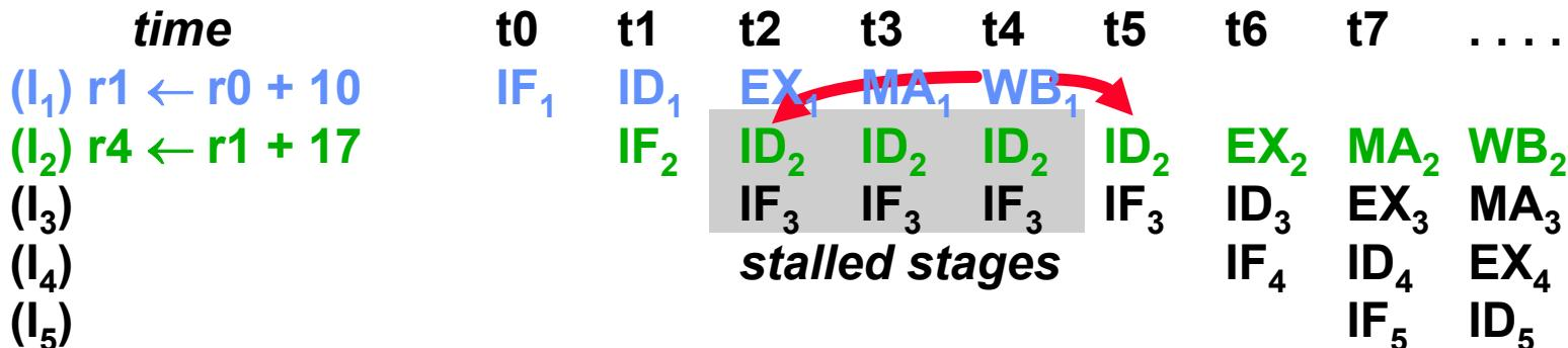
Each *stall* or *kill* introduces a bubble in the pipeline
