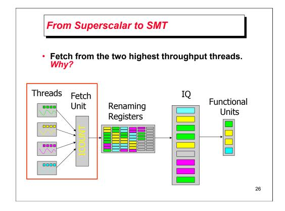
Fetch unit that can keep up with the simultaneous multithreaded execution engine
