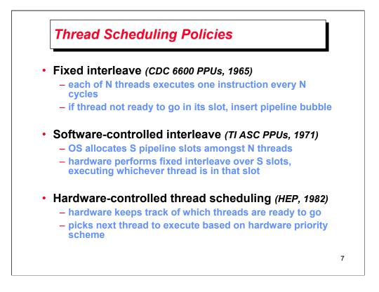
Software-controlled interleave, S > N. Wheel with the threads in each slot. If thread is ready to go
