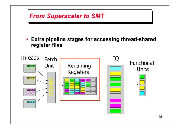
8\*32 for the architecture state + 96 additional registers for register renaming
