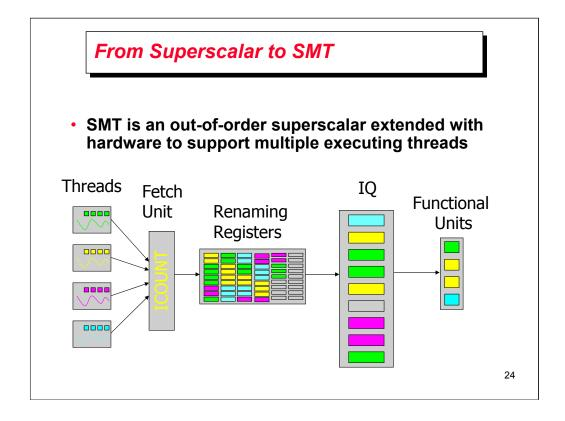
no special HW for scheduling instructions from different threads onto FUs
