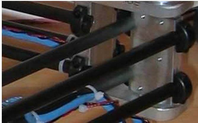
Figure 4-11: Proof-of-Concept 3 – Clamps used to attach carbon-fiber to aluminum.
