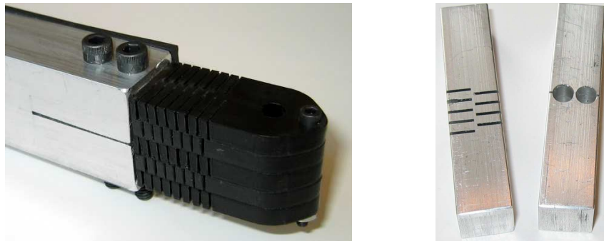
Figure 3-7: Left : Stacked lasercut ABS flexures used for a mechanically compliant arm. Right : Aluminum prototypes of flexures.
