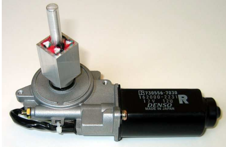
Figure 4-6: Proof-of-Concept 2 – TCEJ mounted on a window lift motor.
