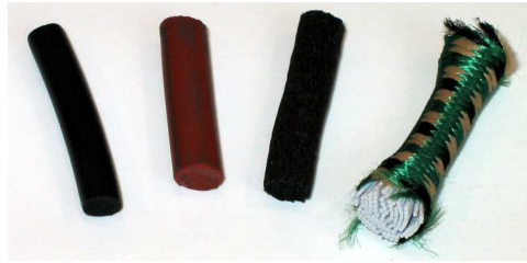
Figure 3-5: Various elastomers used in prototypes of TCEJs. From left to right: Buna-N, Silicone, Neoprene, multi-strand Latex (bungee).
