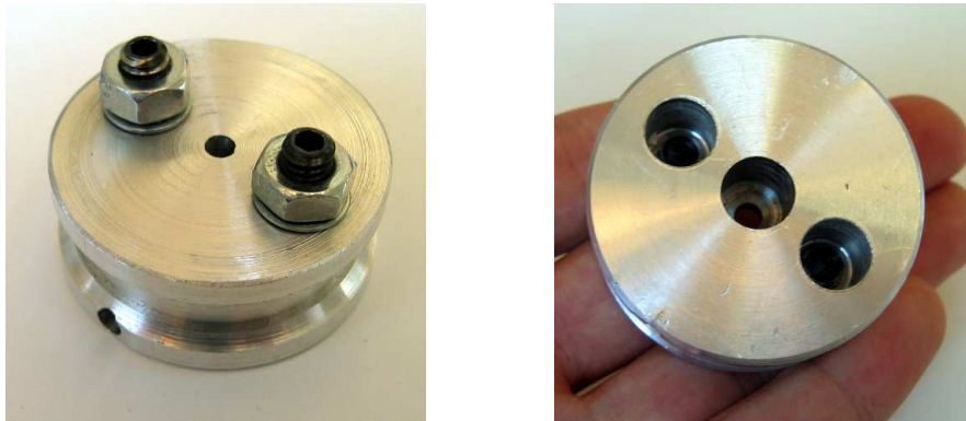
Figure 3-10: Hub with built-in tensioning mechanisms to allow for the large displacement necessary to pre-load a stretchy cable. Left: Top view of hub. Right: Bottom view of hub.
