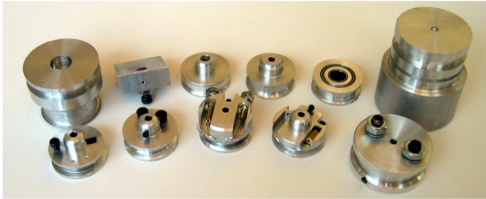
Figure 3-2: A handful of prototypes created to explore various drive hubs with built-in tensioning mechanisms. All of the hubs shown here were designed, fabricated, and tested within a few days' time.
