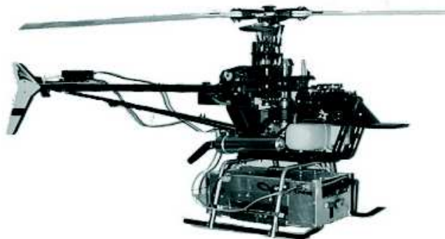
Figure 6-1: MIT's autonomous X-Cell helicopter, equipped with avionics box.
