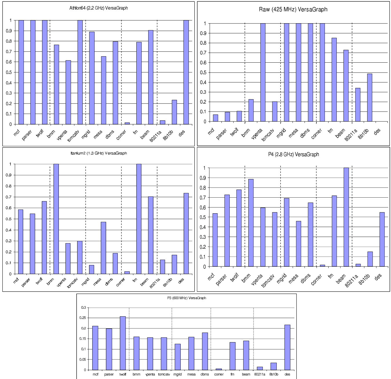
Figure 5. VersaGraphs for five different architectures: Athlon 64 (upper left), Raw (upper right), Itanium 2 (middle left), P4 (middle right) and the P3 (bottom).
