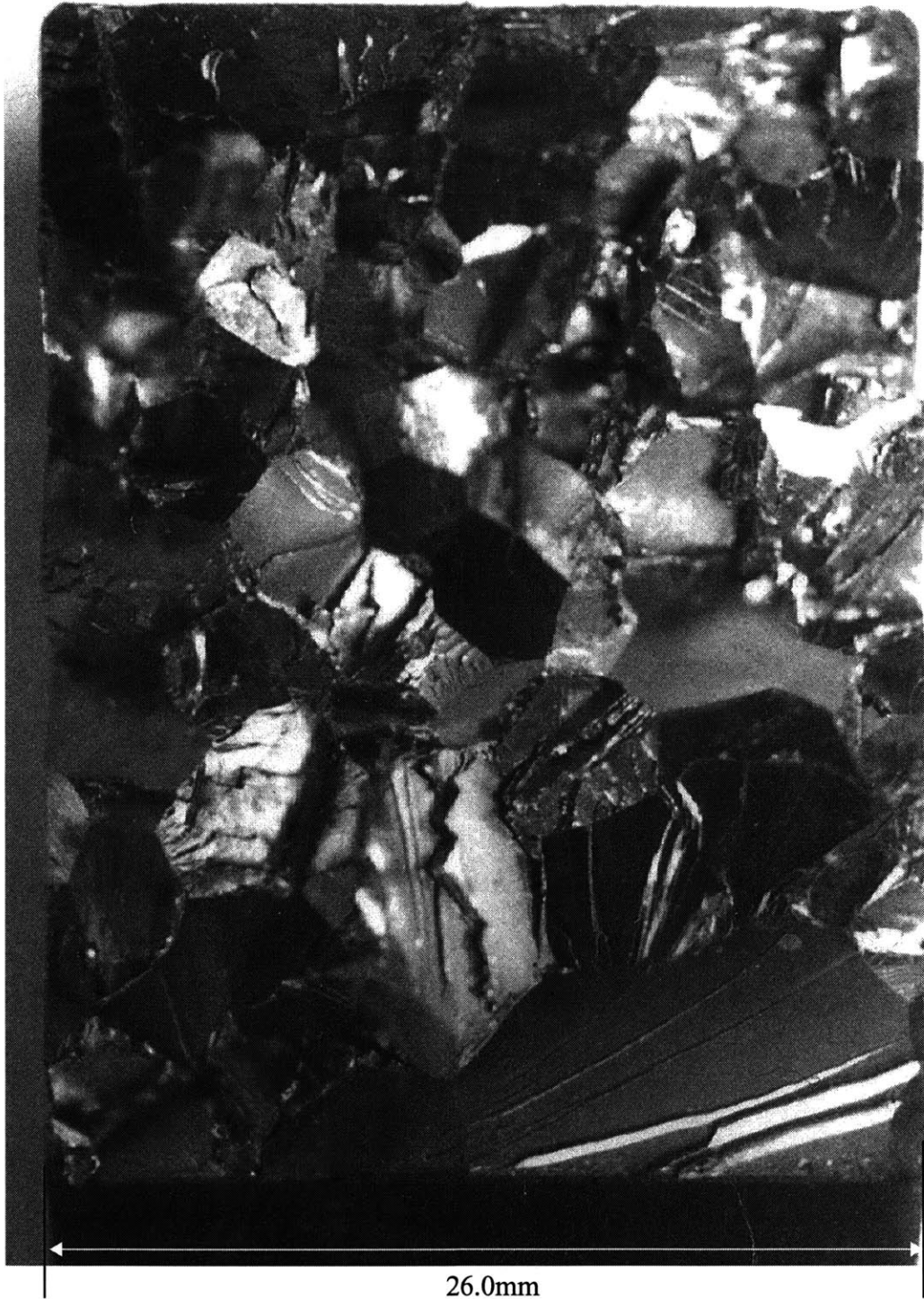
Fig.7-2 Macrograph of a fracture surface of a compact fracture specimen of very coarse grained Fe-2%Si alloy (-30°C).
