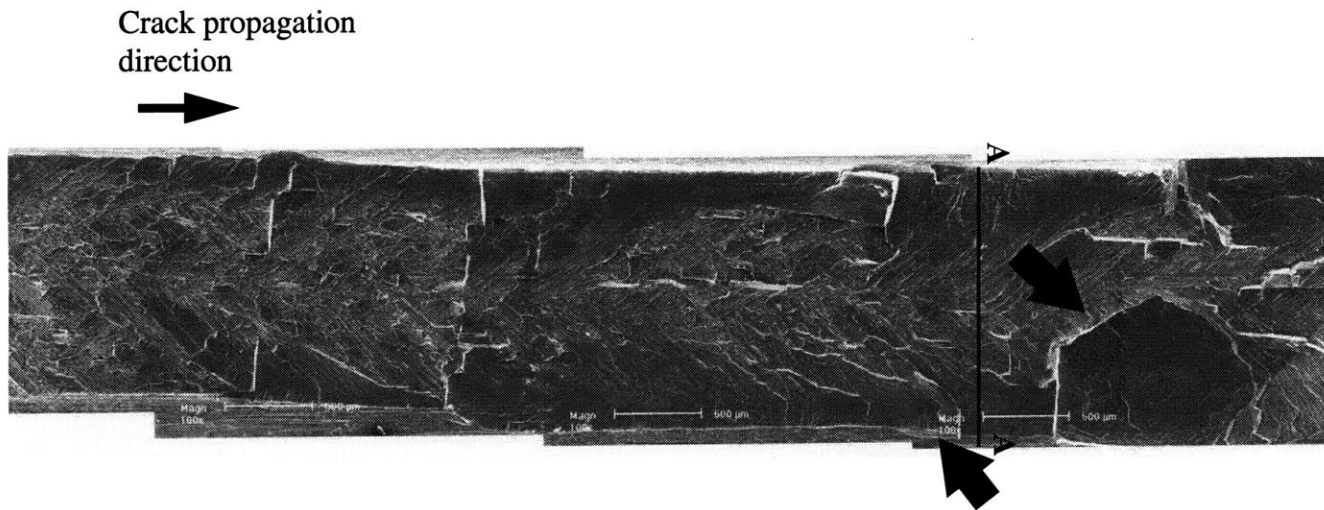
Fig. 4-27 SEM photo of grain A in one of bi-crystal specimens studied in Chapter 2.
