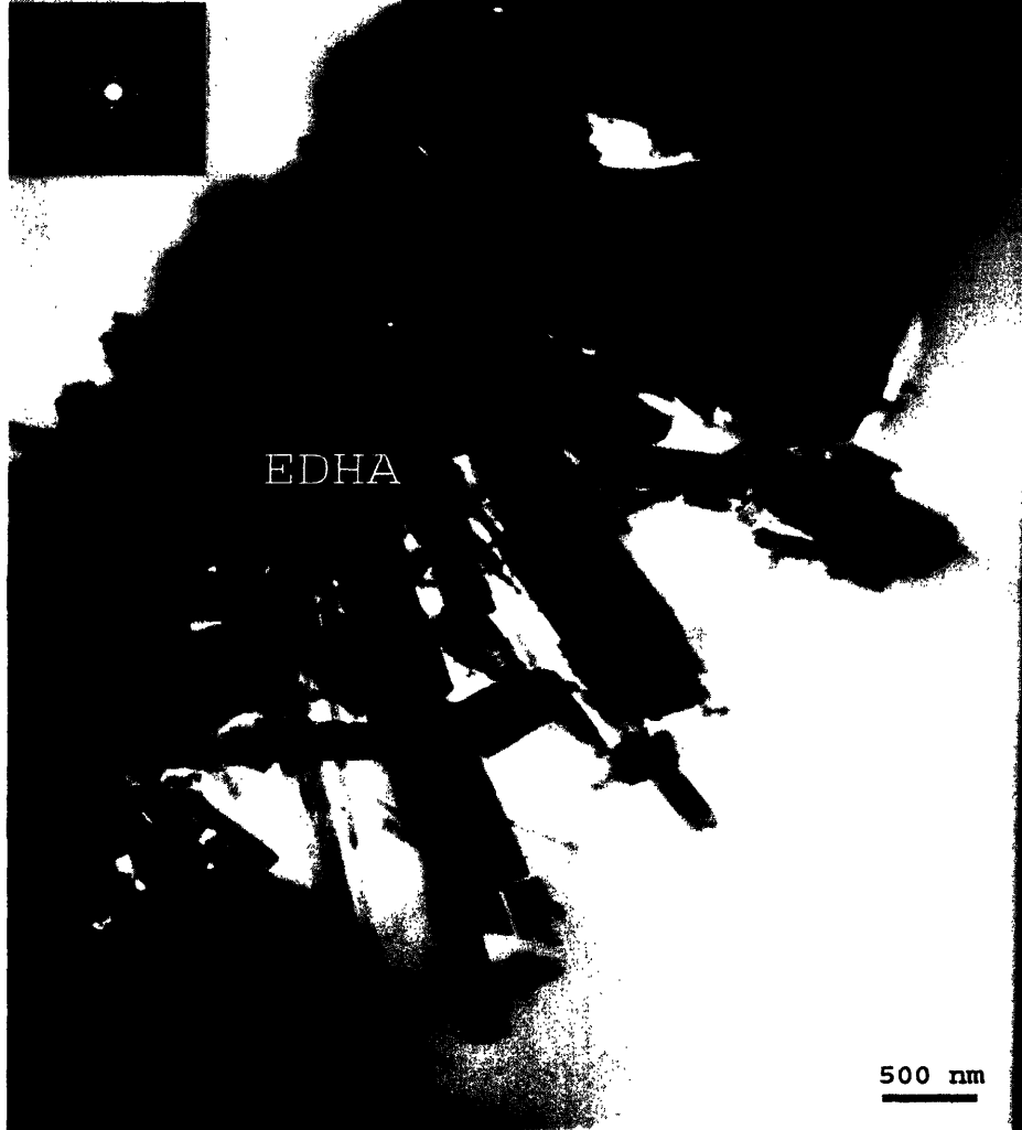
Figure 2-13 Cross-section TEM micrographs of 6-hour EDHA-coated implant showed dendritic growth of the coating. The platelet crystals exhibited single crystal character, by selected area electron diffraction.
