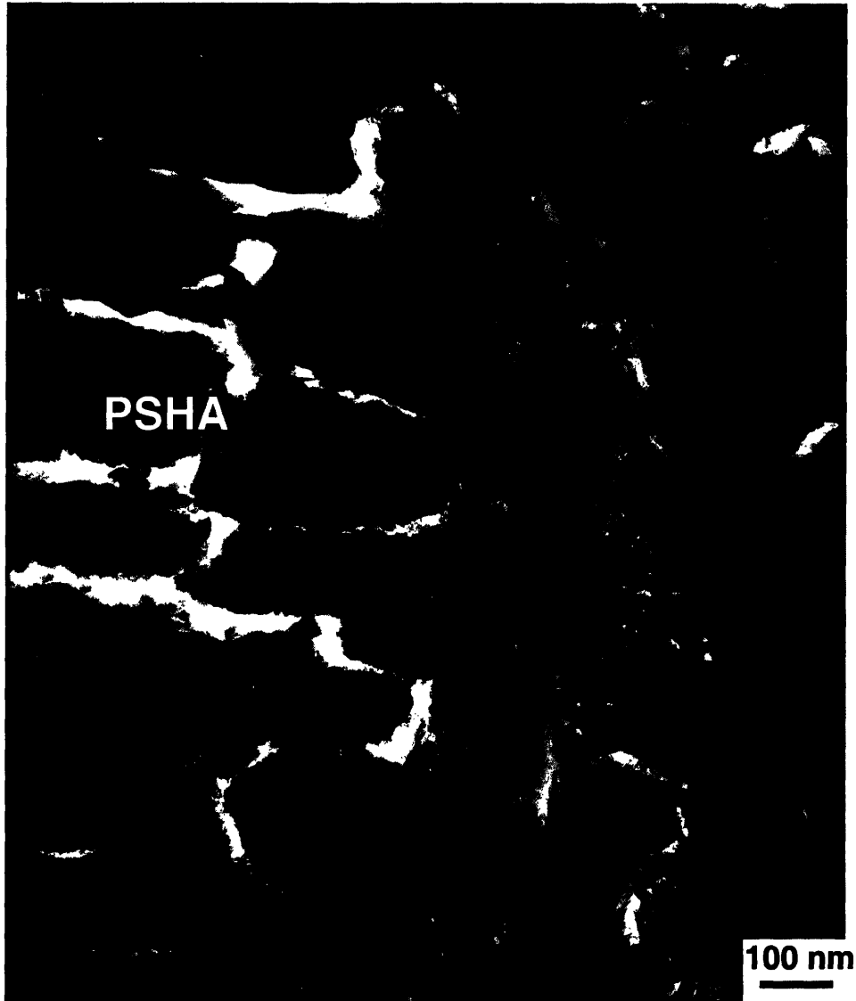
Figure 2-22 TEM micrograph for PSHA coating at 14 days. TEM cross section stained with uranyl acetate and lead citrate.
