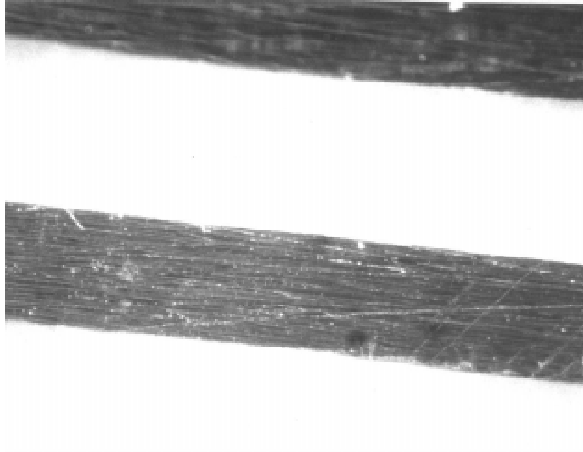
Figure 6.15: Larger magnification optical microscope photograph of the 1 mm wavelength electrodes in Figure 6.14 showing edge sharpness of the Teflon sensor.
