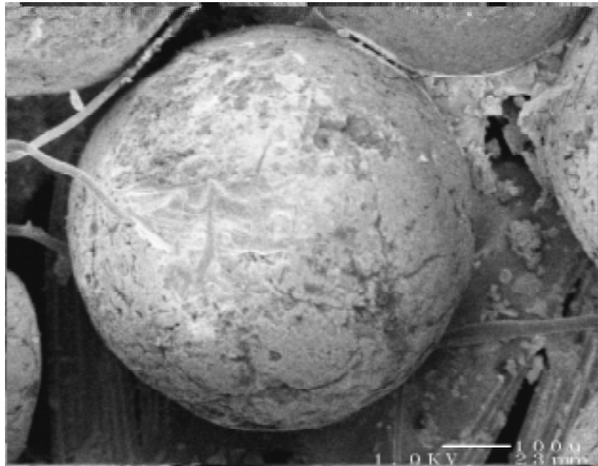
Figure 13.1: An SEM micrograph of the carbon microsphere. The white line is 100 \mu\text{m} (23 mm in the image). Garment fibers are seen in the upper left corner.
