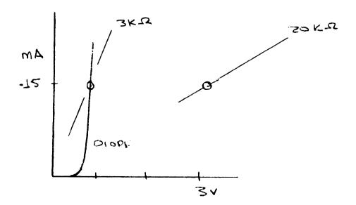
The first log geneator establishes a voltage - current relation based on the diode and 20K resistor.
