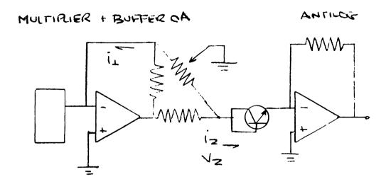
such that  $i_1 = i_2$  and the output voltage of the multiplier is thus controlling the current input to the antilog amplifier transdiode.
