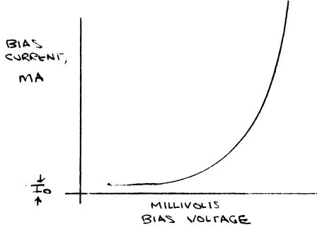
It is important to note that the saturation voltage  $\sqrt{\circ}$  is directly proportional to the absolute temperature.
