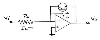
A diode - connected transistor is used to perform the diode function, as transistor emitter-base junctions have more dynamic current range than diodes in general. By the following diagram, an input  $\sqrt{1}$  across RL causes a current flow through the "transdiode". The bias voltage, appearing as  $\sqrt{1}$  varies as the log of  $\sqrt{1}$ .
