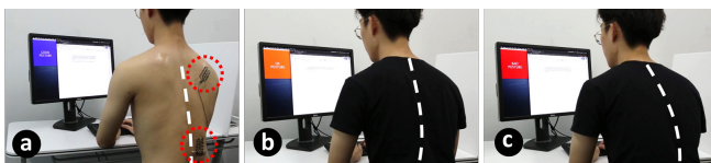
Figure 7. A pair of strain gauge sensors placed on the back are used to sense good (a), moderate (b), and bad (c) postures.
