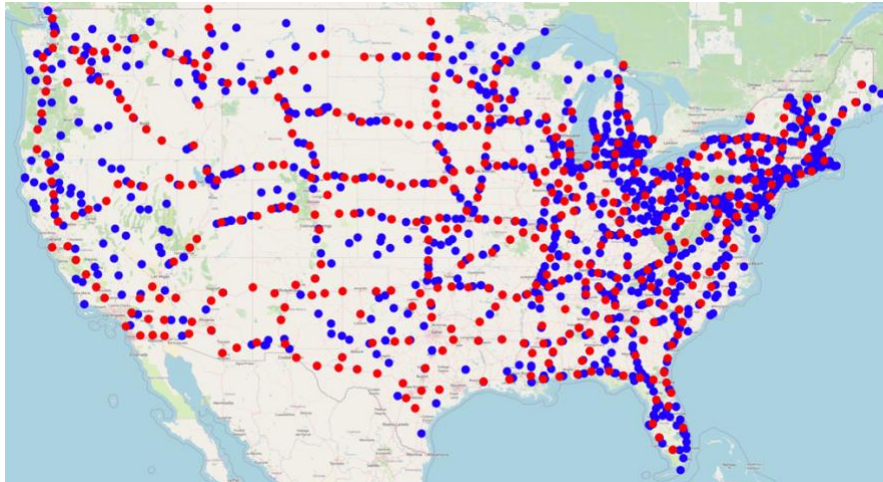
Figure 4.7: U.S. truck stop network before (blue) and after (red) randomly selecting stops separated by 100 miles on average and at least 50 miles
