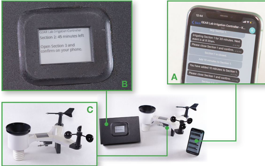
Figure 3-3: The three components of the physical prototype used to facilitate interviews and focus groups. The phone (A) was equipped with a Telegram bot that stepped farmers through a key set of interactions with the tool. The control box (B) displayed the status of these interactions and directed farmers to interact on the phone. The low-cost weather station (C) showed farmers what data the tool might collect: wind speed, wind direction, ambient light, solar irradiance, precipitation, temperature, and humidity.
