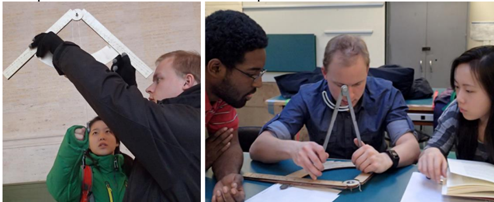
Fig. 9.6 - Sighting (left) and calculating (right) with laser-cut Galileo compass.
