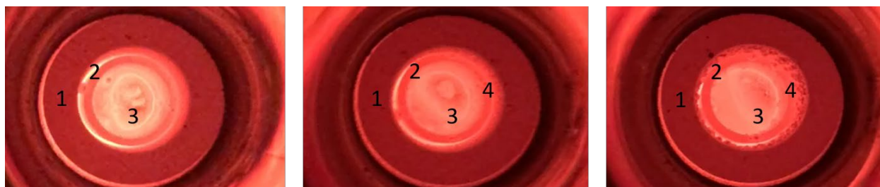
Figure 7.7: View through the top window of an induction furnace fitting during aluminothermic reduction via reactive vacuum distillation. Panels from left to right correspond to the melt upon reaching temperature, after 10 minutes at temperature, and after 20 minutes at temperature. Point 1 corresponds to the graphite susceptor crucible, 40mm in outer diameter. Point 2 corresponds to an inner alumina crucible containing the melt. Point 3 corresponds to the melt with bubble formation due to Al_2S_3 distillation. Point 4 correspond to the buildup of recondensed Al_2S_3 deposit over the course of the experiment higher up on the susceptor outside the furnace hotzone.
