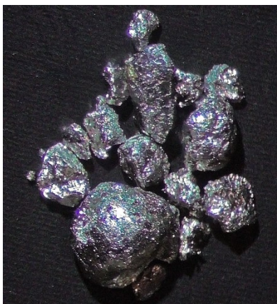
Figure 7.13: Ferrochromium (FeCr) metal droplets produced through aluminothermic reduction of sulfidized chromite ( FeCr_2O_4 ) concentrate via reactive vacuum distillation. Droplets shown are 1-2 mm in diameter.
