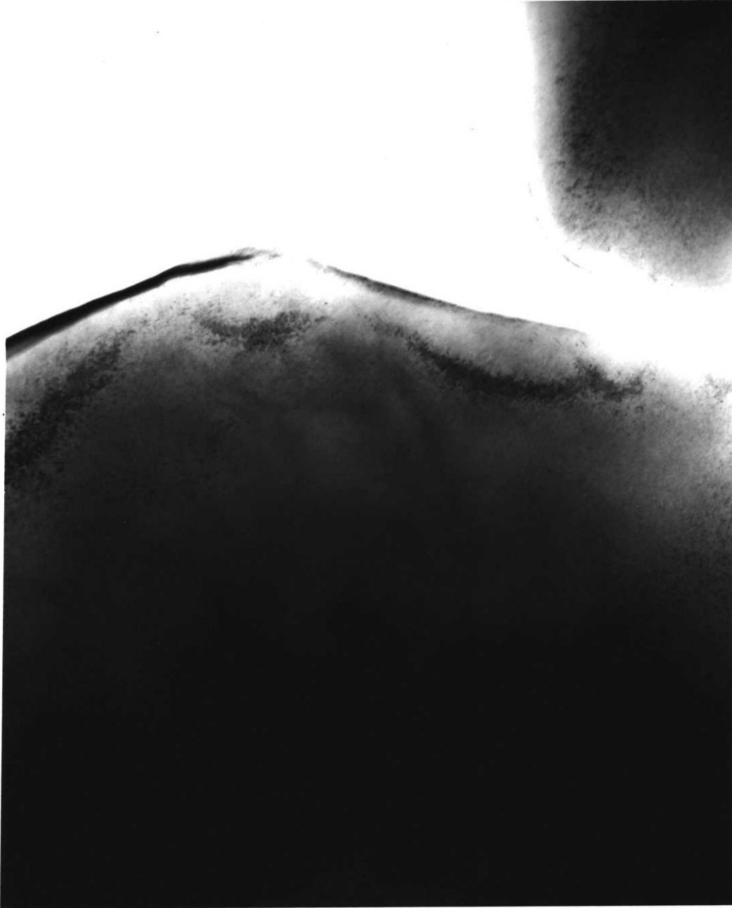
Figure 16 - A transmission electron micrograph of single phase ZrV_2 , showing no structure. Mag. X54,000.
