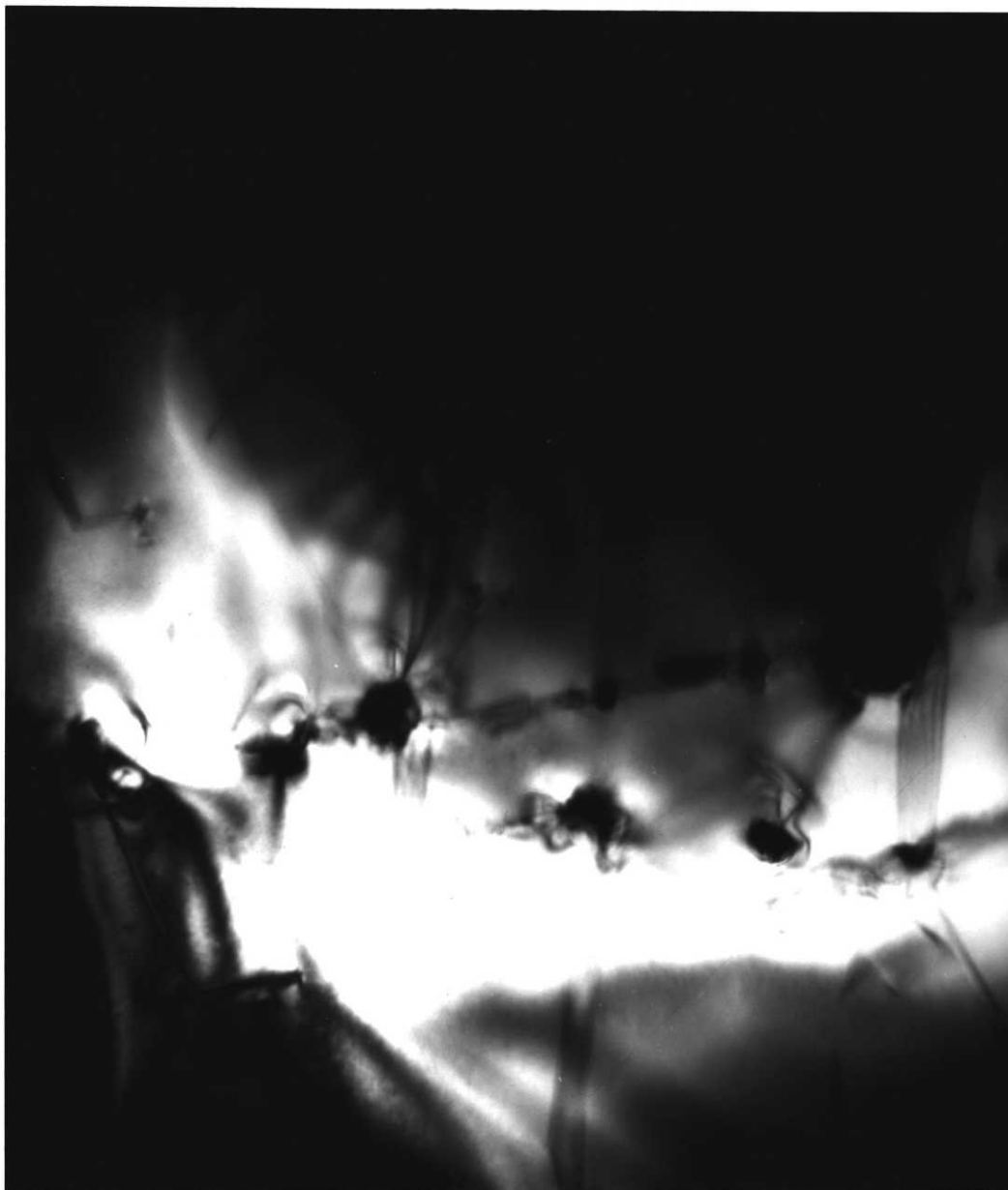
Figure 17 - A transmission electron micrograph of a spark-cut sample showing second phase particles and stacking faults.
