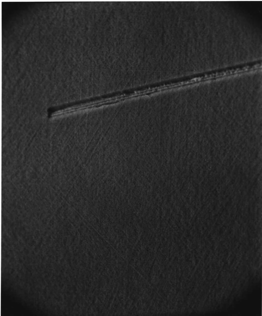
Figure 14 - A scanning electron micrograph of a Zr stringer in the same sample as in Fig. 5, but which has been etched with a different solution. Mag. X2000.
