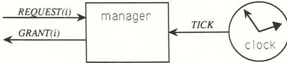
Figure 2: The architecture of the centralized control system.
