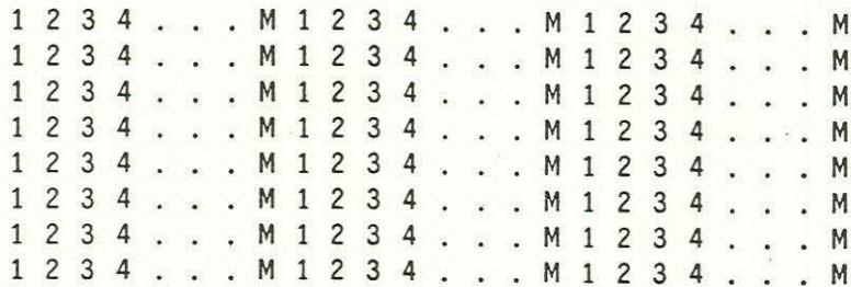
Figure 1. A common organization for raster-graphics memory which is efficient for raster scan, but inefficient for vertical updates.
