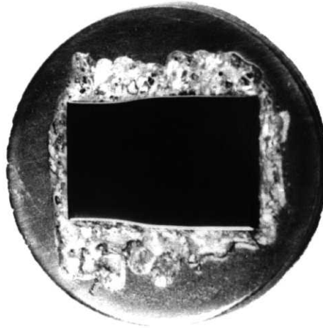
Figure 36. Polished and etched sample mounted on a brass disk with a large ohmic back contact (see text),
