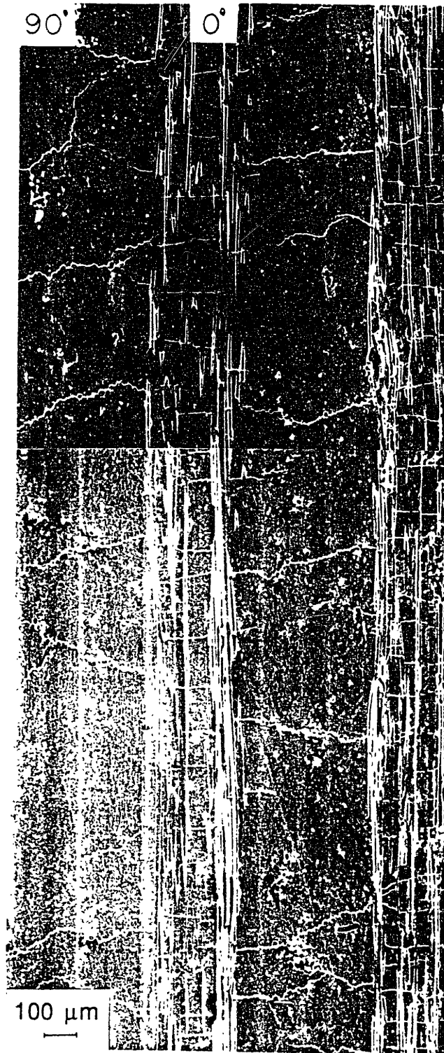
Fig. 4-30 Edge replica of crossplied Nicalon/CAS-II following tensile loading to 0.5 % strain at room temperature.
