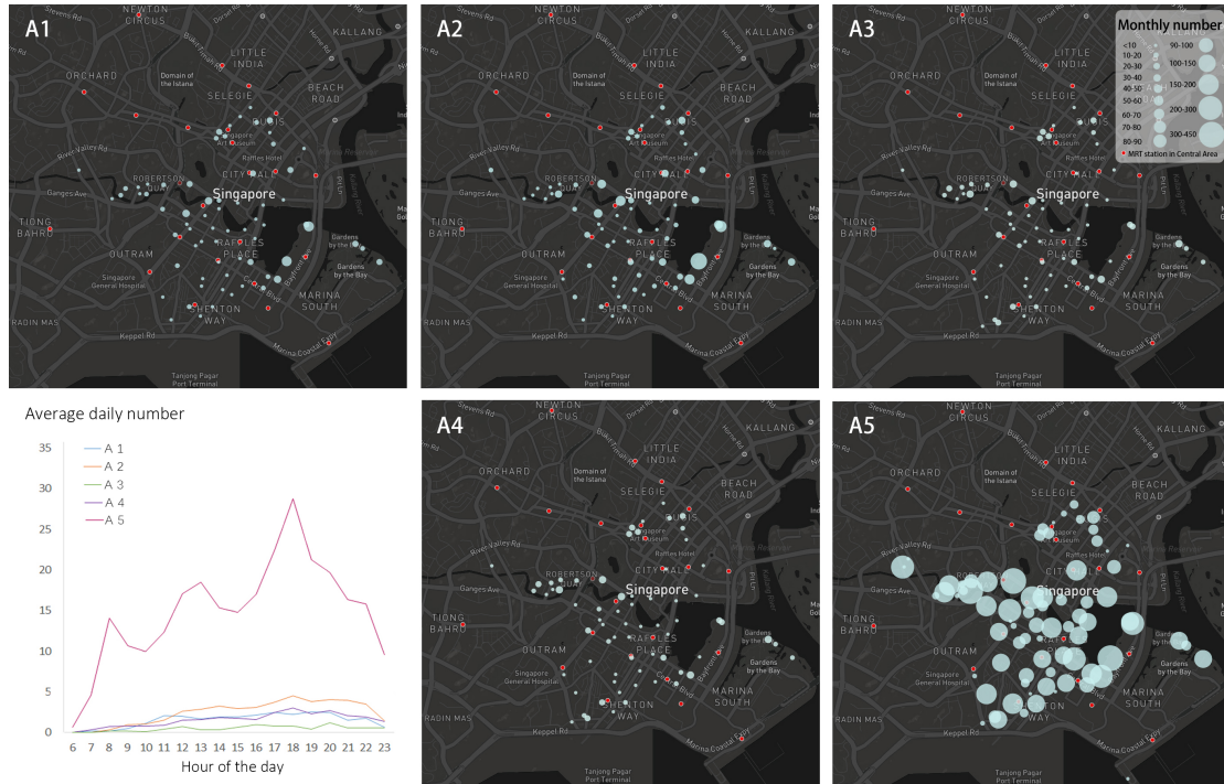
Fig. 7. Numbers of travel demand under A1-A5 e-scooter services: average daily number in hours of the day and monthly number aggregated at origins (e-scooter starting parking locations)
