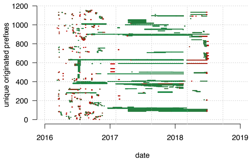
(b) Serial Hijacker AS: Prefix origination of AS3266 (Bitcanal) over the course of 3 years. This AS announces a large number of prefixes over short time periods.
