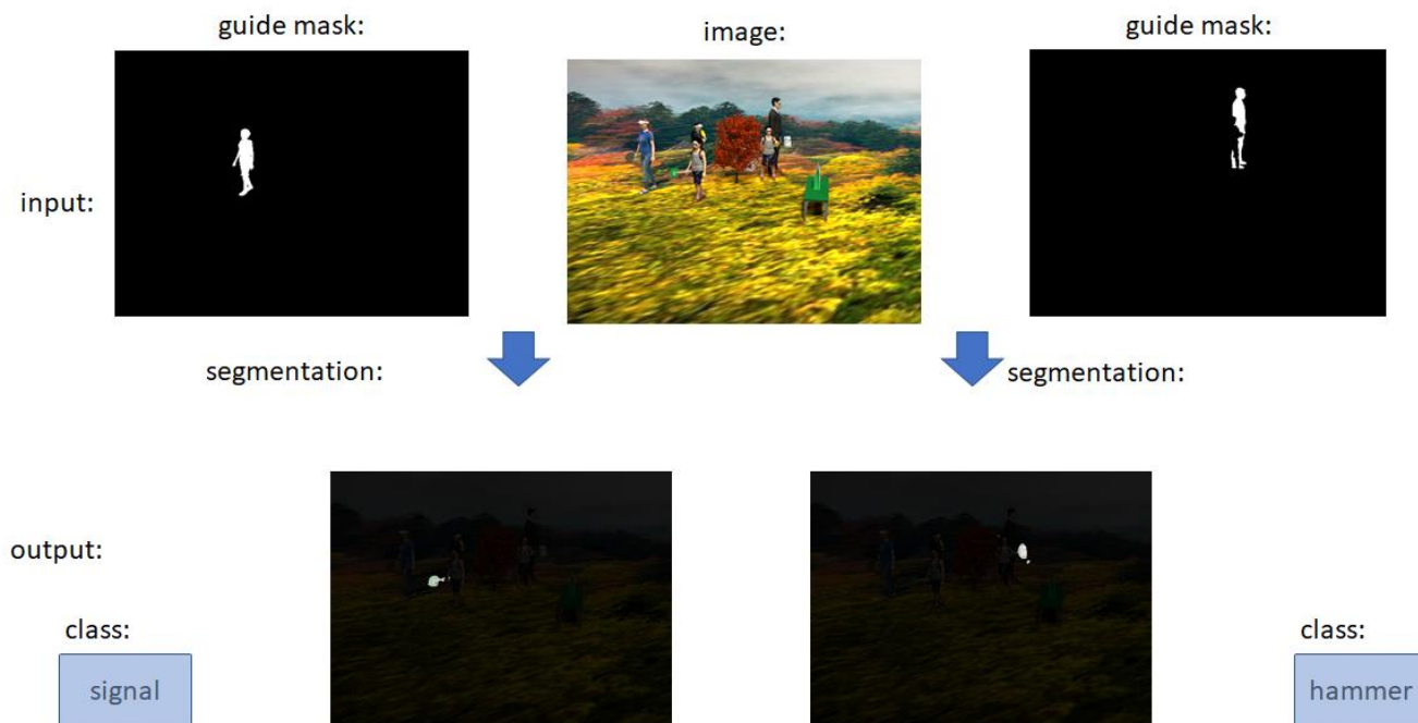
Figure 12: Holding Extracting two ‘holding’ relations from the same scene. Top row shows the input, the scene image and the guiding masks of the reference persons for the relation. Bottom row shows the segmentation maps of the held objects
