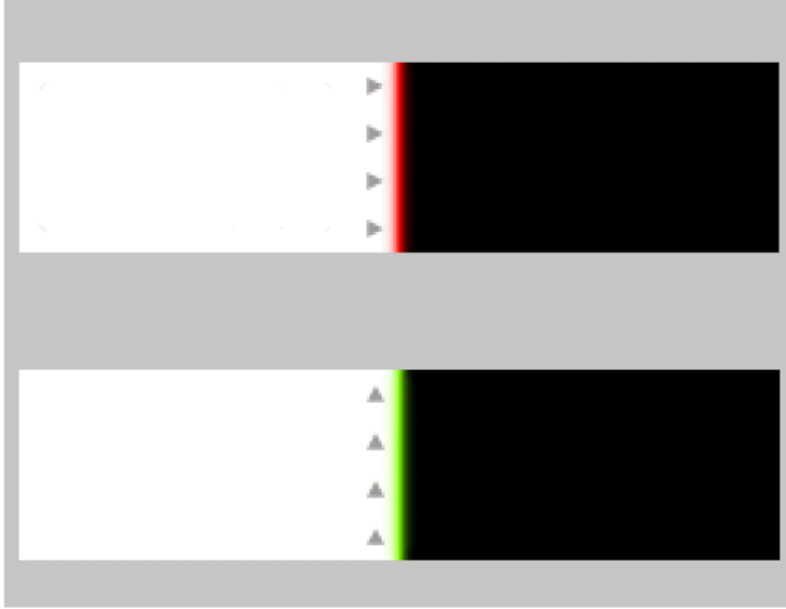
Figure 1.9: Micromagnetic simulations of Néel (top) and Bloch (bottom) domain walls in a magnetic strip. The simulations parameters are the same as those used in Thiaville et al. 50
