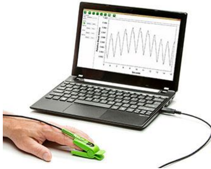
Figure 4.5: QuantaFlo™ sensor connected to a laptop while the software processes the measurements to produce an ABI. [23]
