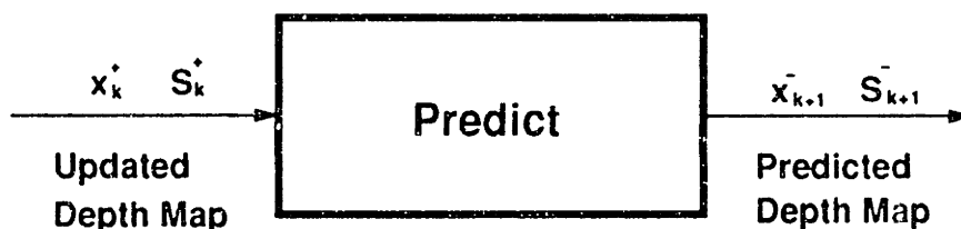
Figure 5.3: The prediction stage of the Kalman filter for temporal surface reconstruction.
