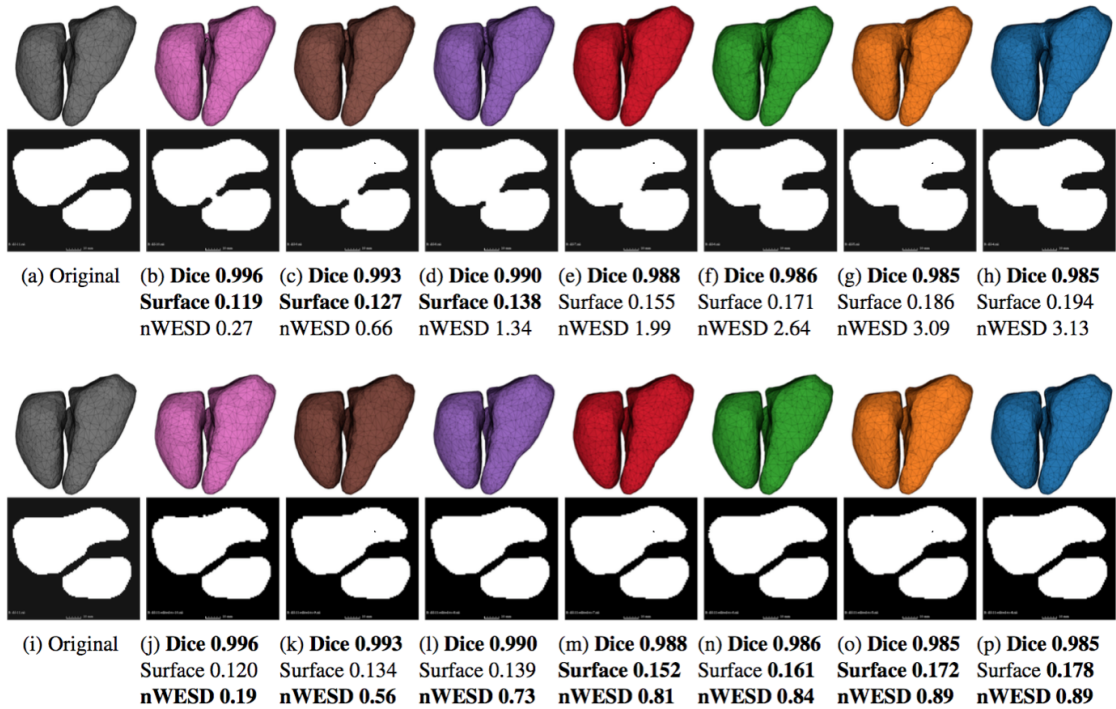
Figure 5-1: Comparing image segmentations of the heart’s two ventricles illustrates the deficiencies of the Dice score and average surface distance, and the advantages of a spectral shape similarity measure (nWESD [191, 192]). The segmentations in the top and bottom rows have the same number of incorrect pixels, even though those on the bottom are intuitively much better. For each column, bold scores indicate higher similarity to the original segmentation on the left.
