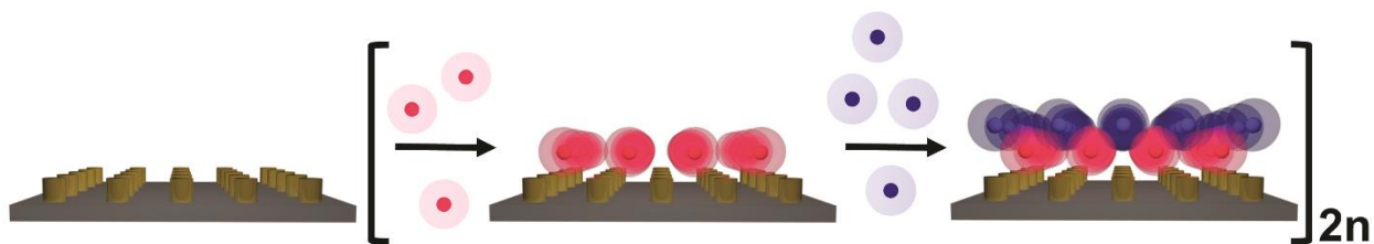
Scheme 3.1: Layer-by-layer assembly of PAE superlattice thin films on a DNA-functionalized template.
