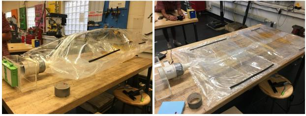
Fig 3-1: Generation 6 SurgiBox prototype shown in inflated state (left) and deflated state (right).
