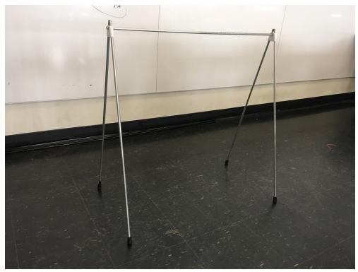
Fig 5-7: Assembled A-frame support frame
