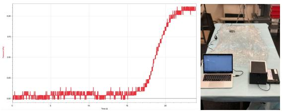
Fig 5-2: Sample data of the filter surface area experiment, the graph shows pressure as a function of time.. The time to inflation is measured from when the slope first begins to increase, to when the slope decreases back to zero.
