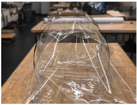
Fig 5-13: Spring steel frame in TPU enclosure, axial view.
