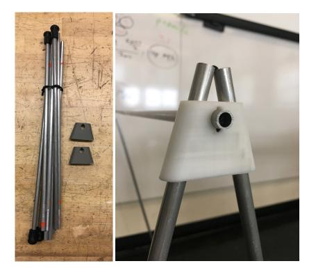
Fig 5-8: A-frame support frame in packed configuration Fig 5-9: Detail of plastic components on support frame
