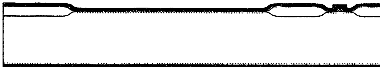
Figure B.18: LPCVD silicon nitride deposition.
