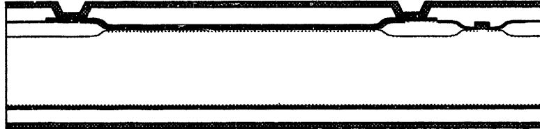
Figure 3.5: LPCVD polysilicon diaphragm deposition, phosphorus doping, and glass wet-etch.
