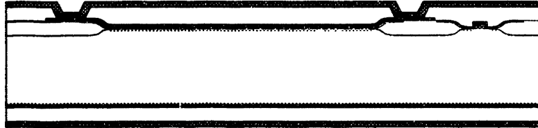
Figure B.21: LPCVD polysilicon diaphragm deposition, phosphorus doping, and glass wet-etch.
