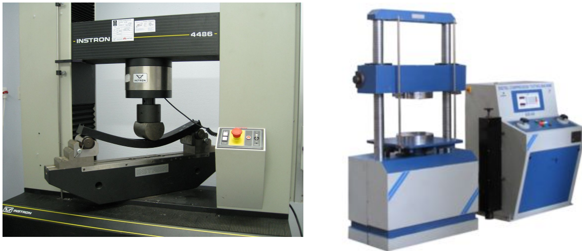
Figure 13: The machine on the left is a three point bending machine and on the right is a compression machine which we were not able to apply
