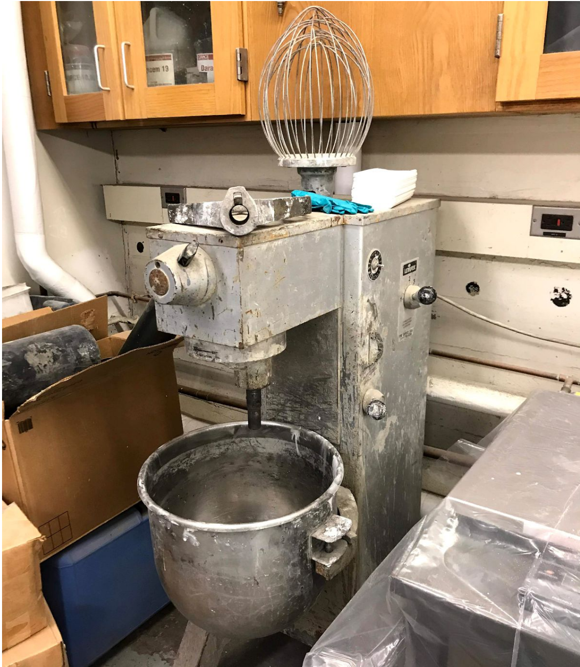
Figure 8: Hobart Mixer we used to mix the materials
