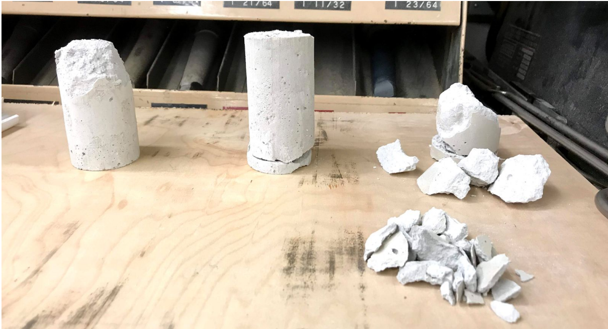
Figure 22: From left to right, Batch 8 [400g water], Batch 9 [300g water], Batch 7 [500g water]
