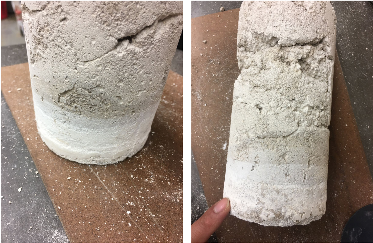
Figure 15: Professor Linn Hobbs' Cylinder right after demolding
