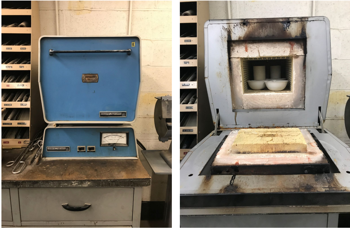
Figure 12: Furnace used to bake quicklime at 1100°C and oven curing of samples at 600°C for 4 hours
