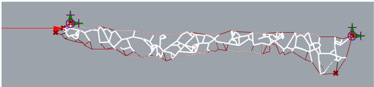
Figure 8. Lateral wind load applied to the left side of the web geometry structure.
