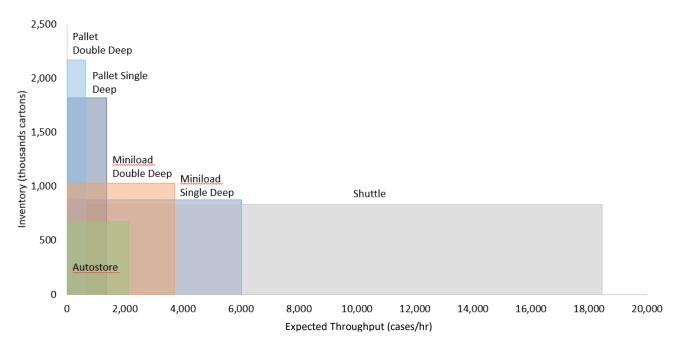
Figure 21: Expected throughput and inventory capacity of different ASRS in a 500' x 300' x 60' building.
