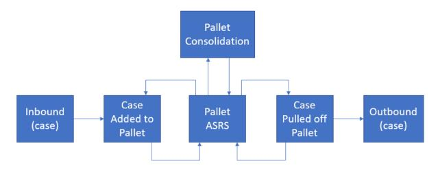
Figure 20: Pallet case flow
