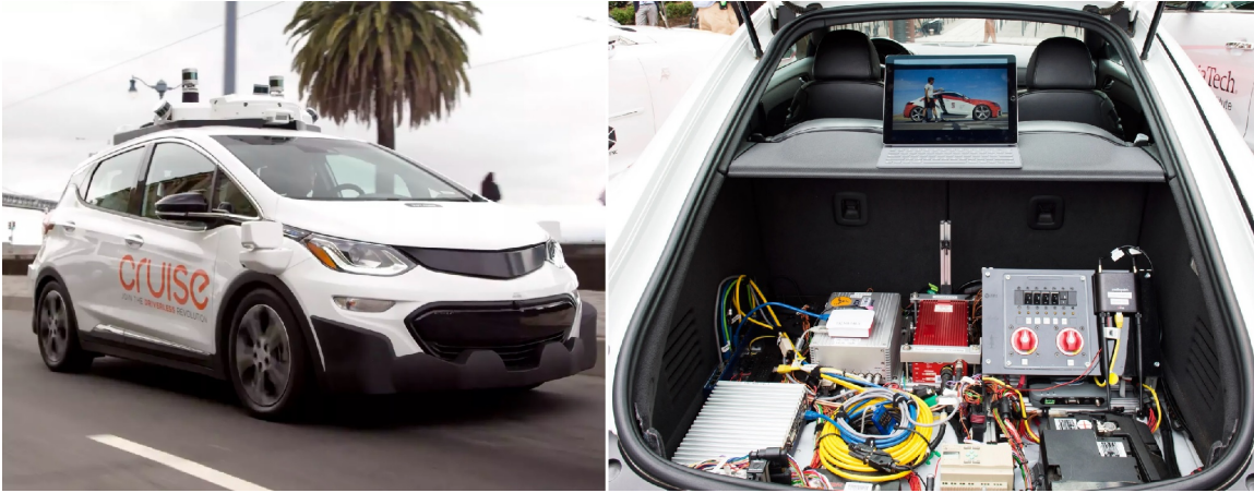
Figure 8-1: An autonomous crown on a GM Cruise and a trunk on a Stanford Univ Audi AV with an autonomous compute stack
