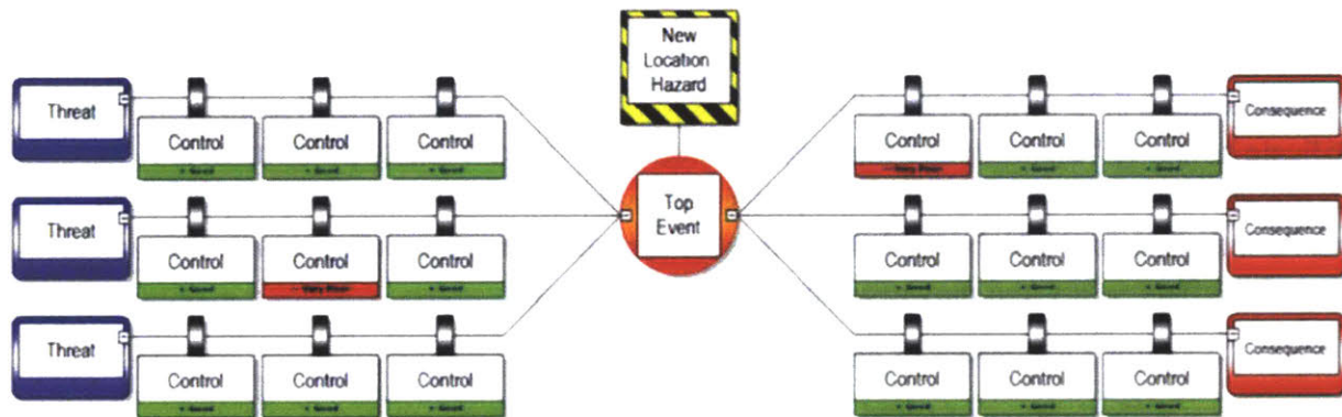
Figure 6. Structure of the Bowtie model (CAA UK, 2019)
