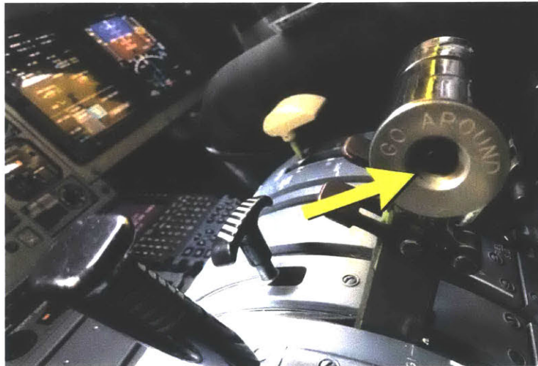
Figure 28. Throttle pedestal in commuter aircraft
