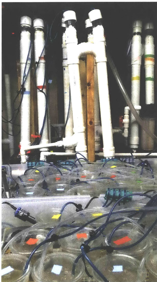
Figure S1. Acidification and egg culture system. Filtered, temperature controlled water from Vineyard Sound was piped into a header tank (behind PVC towers depicted) and flowed into PVC towers where airstones equilibrated water to the desired p\text{CO}_2 levels. Water exiting the chamber was split in a manifold (not depicted), which fed drip lines into the egg culture cups of each water bath
