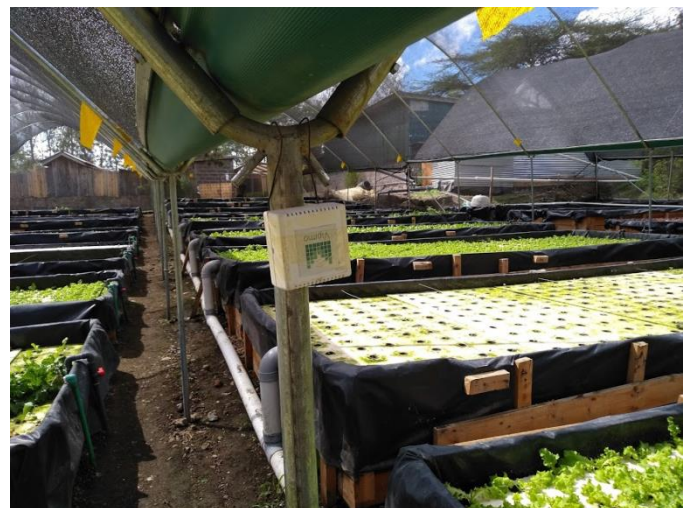
Figure 12: A Upande Vipimo T/RH sensor in the aquaponics greenhouse at Kikaboni Farm
