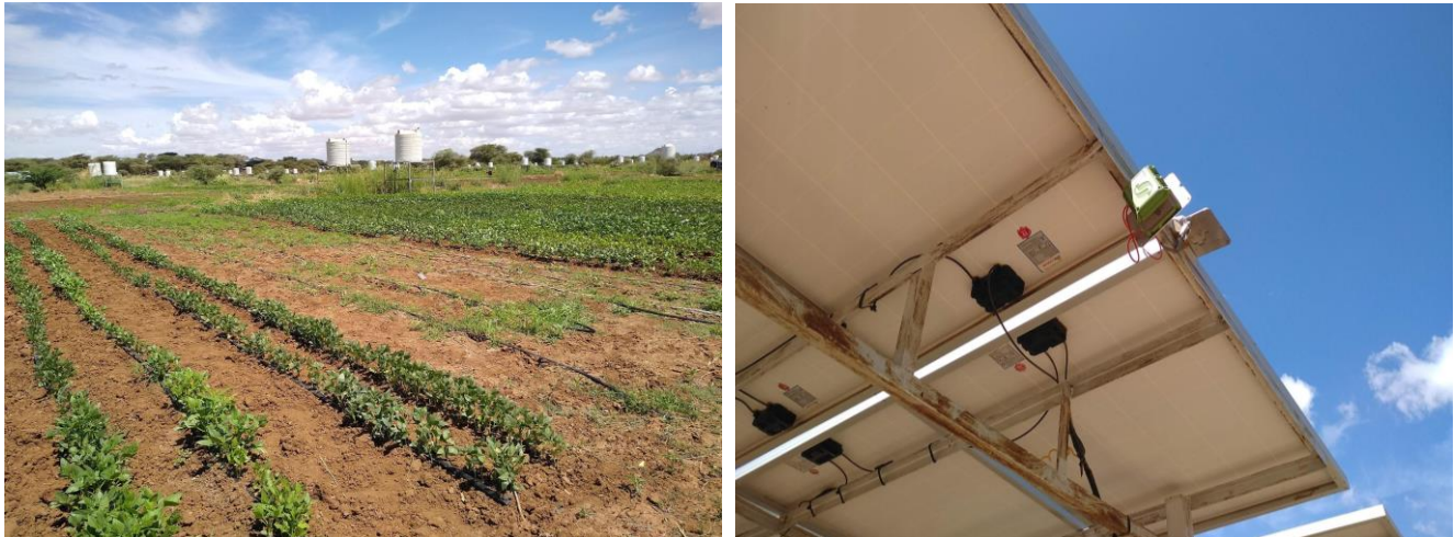
Figure 17: Drip-irrigated vegetable cultivation at Napuu 1 Drip Irrigation Scheme in Lodwar, Kenya (left), and a SweetSense gateway mounted on solar PV panels that transmits solar irrigation pump usage data to an online server via cellular or satellite data (right)
