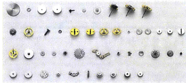
Figure 7: Complicated, but not complex – Grand Seiko Spring Drive watch components [16]
