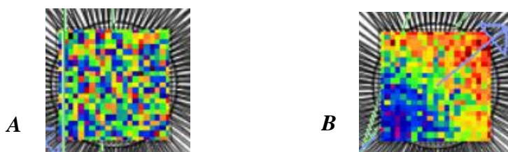
Fig. 5, Substrate planes showing pressure variations after approx. 10 min of simulation with the source A in its original position B with a 100mm extension; Max/Min (mbar): A 1.91E-05/1.57E-05 B 2.93E-05/1.66E-05
