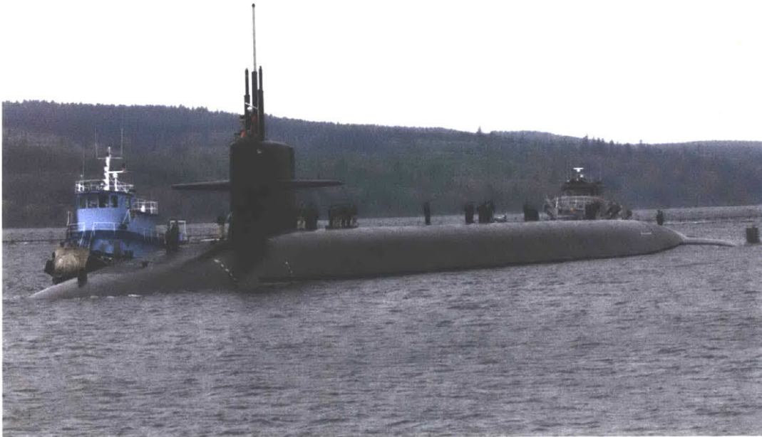
Figure 13: Ballistic Missile Submarine Superstructure ("Turtleback")
