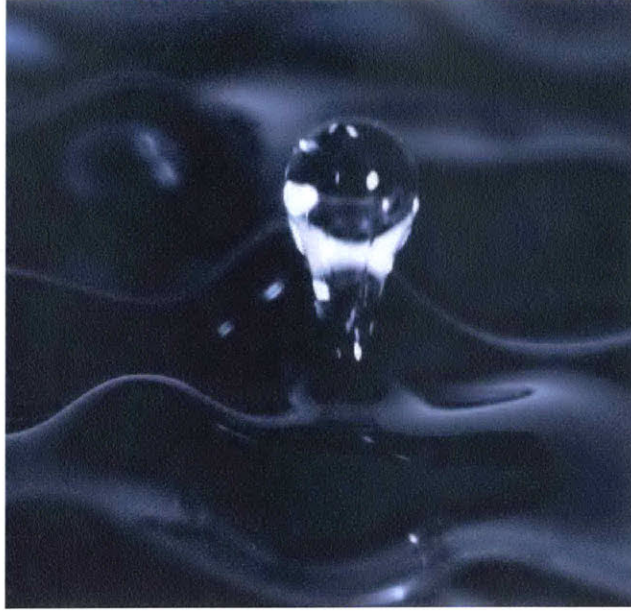
Figure 4-3: Faraday wave rupture generates drops when the vibrational acceleration is sufficiently high, \gamma > \gamma_R ( = 4.02\gamma_F for 20 cS oil vibrated at 80 Hz).
