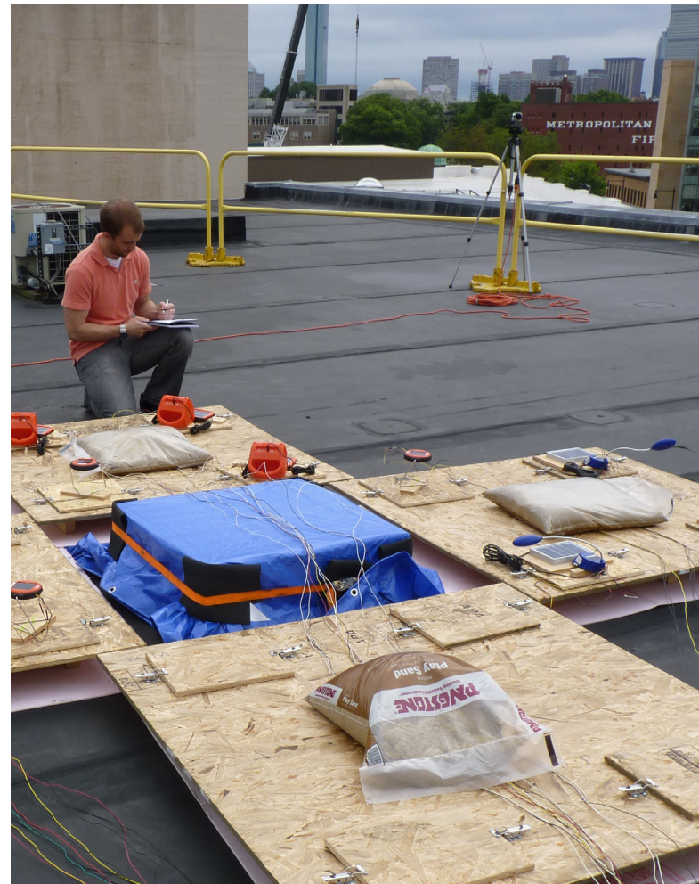
(Top) MIT Lantern roof exposure: During the summer of 2013, CITE was able to charge up to 16 lanterns by exposure to the Boston sun using one of MIT's rooftops. From sunrise to sunset, the solar radiation was monitored for its intensity by a radiometer. This measure of incident radiation was used to determine the efficiency of the lantern's solar panels in bright sun or when there was a cloudy overcast. The time to charge and discharge were analyzed to give a measure of lantern usefulness where a long time to charge and/or a short time to stay lit makes it less useful to a consumer. Photo taken by Jeff Asher.
